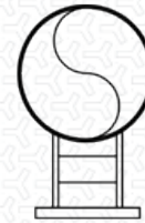
FIGURE 3200 Welded onto the pipe.
