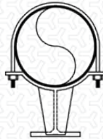
FIGURE 3110 / 3111* Fabricated with two cradles and comes with two u-bolts to hold the pipe in place. Gusset plates provide extra support.
