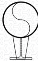
FIGURE 3100 Welded onto the pipe and has gusset plates to provide extra support.
