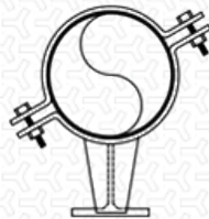
FIGURE 3120 / 3121* Fabricated with two clamps to hold the pipe in place and has gusset plates to provide extra support.
