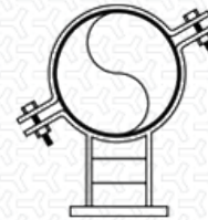
FIGURE 3220 / 3221* Fabricated with two clamps to hold the pipe in place.
