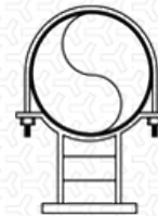
FIGURE 3210 / 3211* Fabricated with two cradles and comes with two u-bolts to hold the pipe in place.
